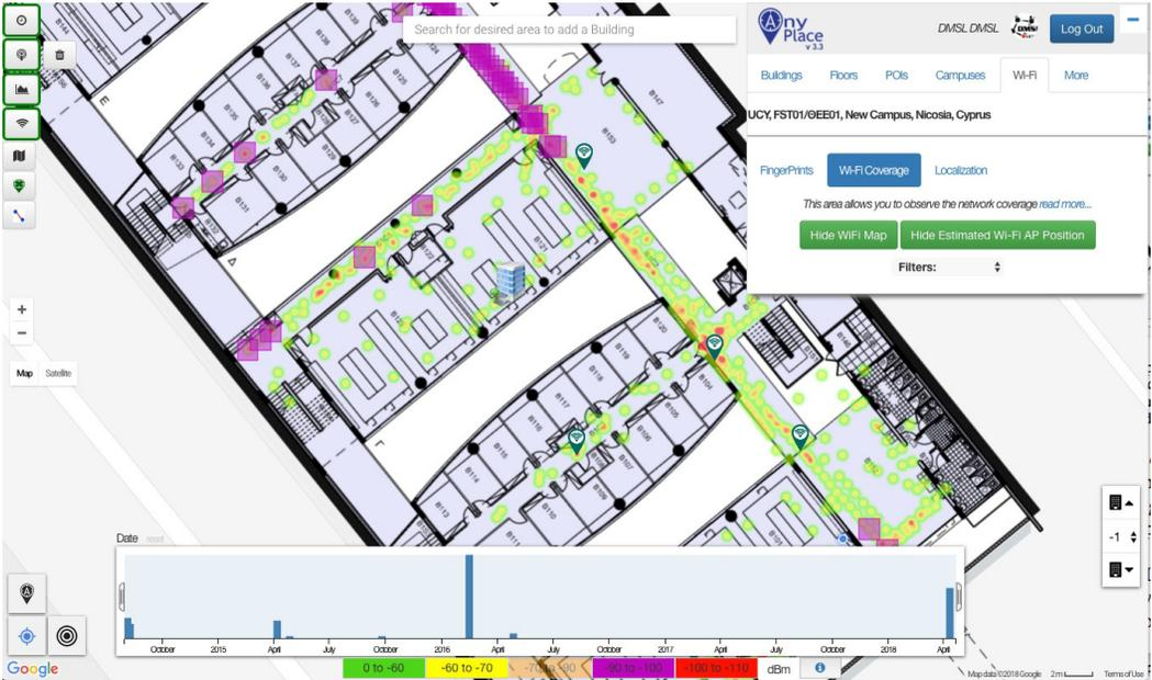
Fig. 7. The Fingerprints Management Studio (FMS) provides a spatio-temporal platform to: (i) manage the collection of location-dependent *fingerprints* in indoor environments; (ii) estimate the localization accuracy based on the collected fingerprints; and (iii) assess Wi-Fi coverage and data rates.
