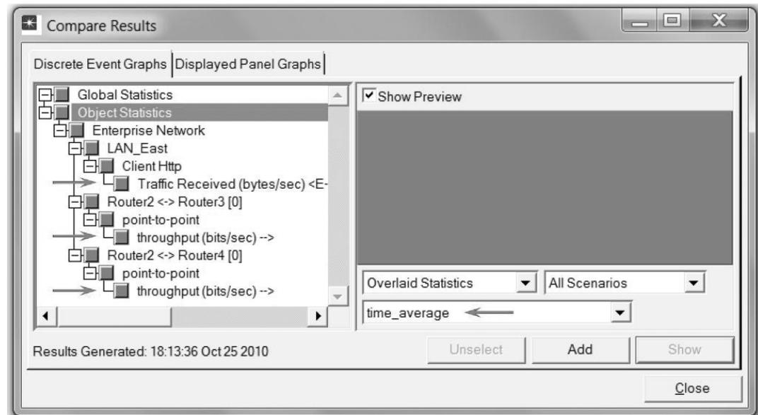
3. Select and show the graphs of the statistics shown previously: **Traffic Received in LAN\_East**, **throughput in the Router2-Router3 link**, and **throughput in the Router2-Router4 link**. The resulting graphs should resemble the graphs that follow.
