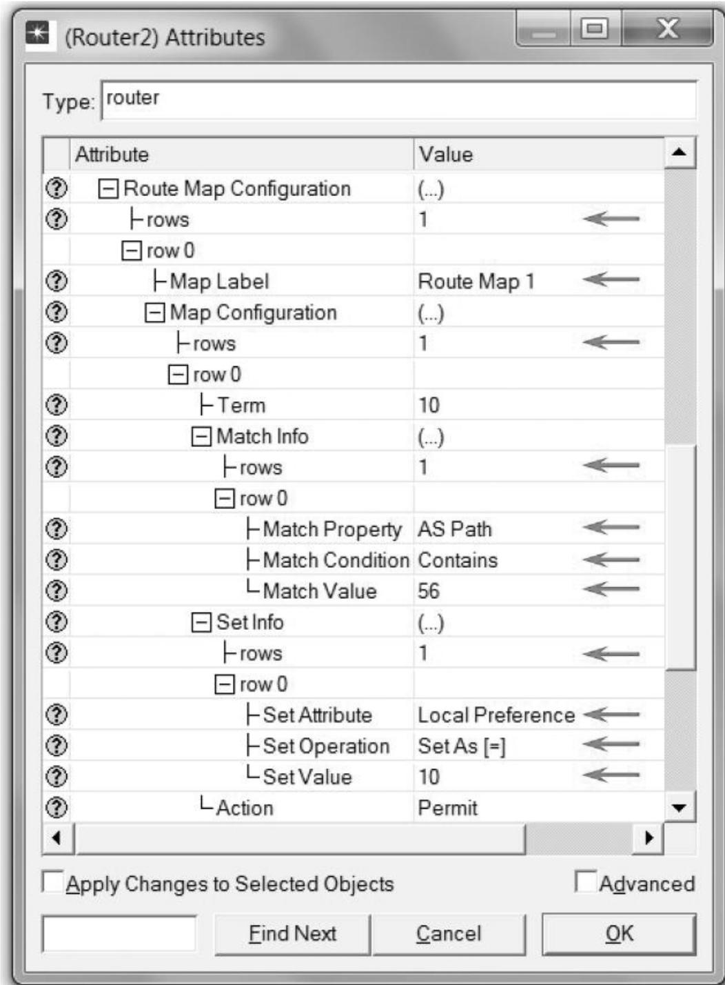
The next step is to assign the preceding route map to the link connecting Router2 to Router3. This way traffic from Router2 to AS 56 will be preferred to go through Router4 instead.
