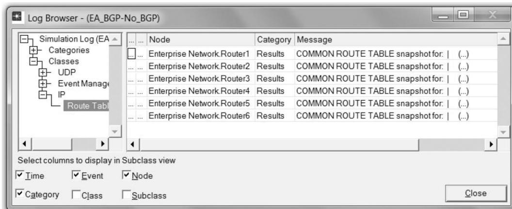
2. Carry out the previous step for scenario **BGP\_Simple** by clicking **Ctrl + 2** at the beginning. The following are partial contents of **Router2's** routing table for both scenarios. (Note: Your results may vary due to different node placement.)
