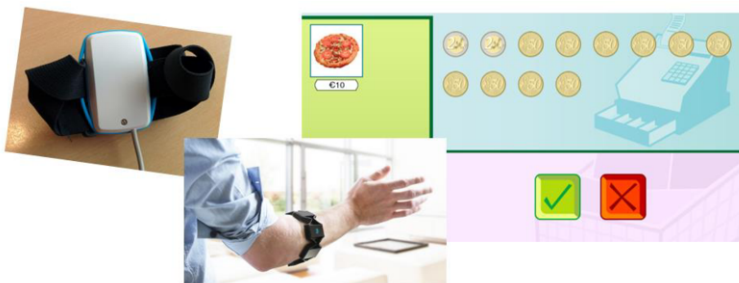
Figure 8. Controlling the EURO application with simple wrist movements - for people who are not able to control their hands or feet with precision.
