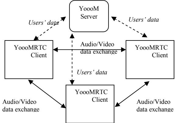
**Figure 2. YoooMRTC Module Architecture**
