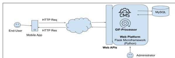
**Figure 2: ASM4Deaf System Architecture**
