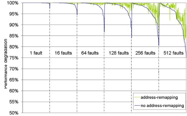
Fig. 7. Remapping vs. No Remapping.
