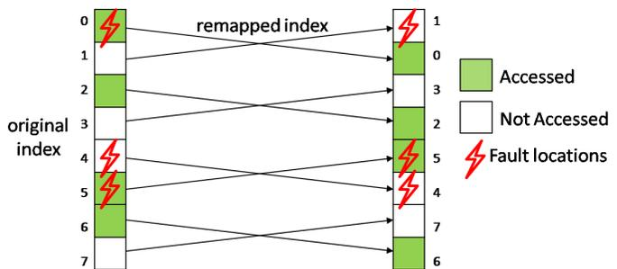
Fig. 2. *Principle of address-remapping.*
