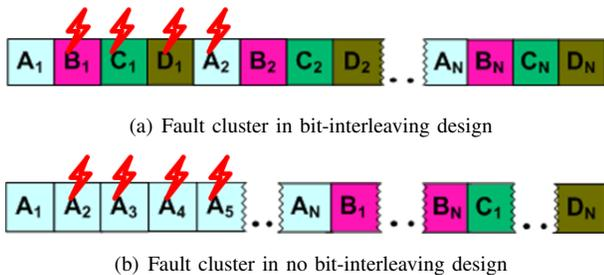
Fig. 1. *Bit-Interleaving vs. No Bit-Interleaving with multi-bit faults.*
