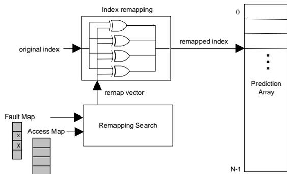
Fig. 3. Prediction Array Protection Scheme.
