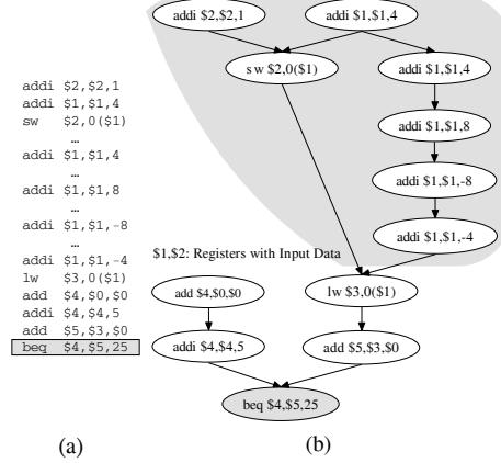
**Figure 1. (a) Example Dynamic Sequence, and (b) the Component-Graph for a Branch Instruction**
