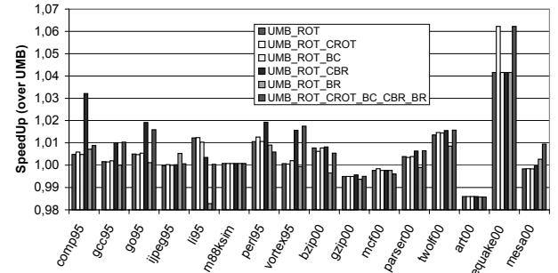
**Figure 9. SpeedUp with various combinations of transformations**
