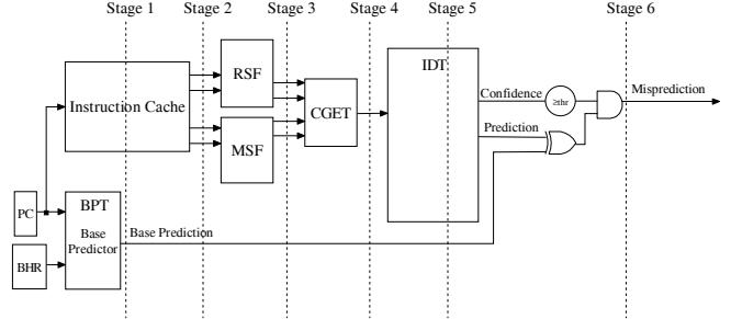
**Figure 5. Pipeline with an Overriding Isomorphic-Based Branch Predictor**
