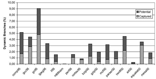
**Figure 8. Mispredictions not Overridden due to Confidence Estimation**
