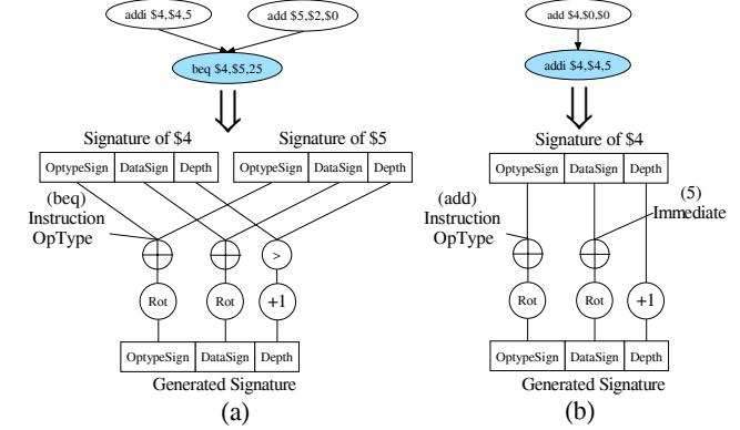
**Figure 4. The Encoding Procedure (a) Commutative Instruction, and (b) One input instruction**
