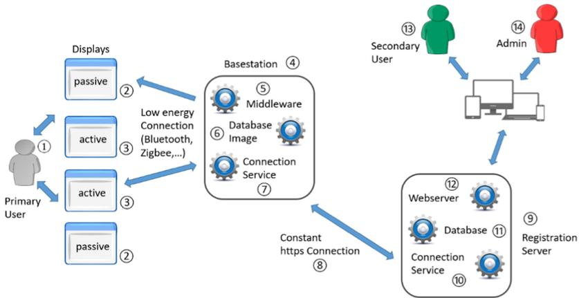
**Fig. 1.** High-level system architecture
